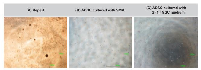
Both SCM and SF1 hMSC Medium expanded adipose tissue MSCs showed no tumorigenic potential in vitro as indicated by anchorage independent soft agar colony formation assay. Colony formation was observed in Hep3B as a positive control. Cells (5x10³) were seeded in 24-well plates and the average numbers of colonies from five independent fields were determined on day24. Hep3B(A) shows 10 colonies, ADSC cultured with MSCs SCM (B, P11) and ADSC cultured with SF1 hMSC Medium (C, P1+10).
